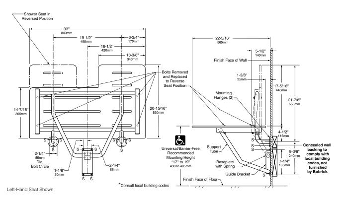
**Installation to Wall.** Secure unit to wall at points indicated by an *S*, with the two Mounting Flanges located at top and the Baseplate and Guide Bracket below. The bottom of the Support Tube must be positioned within the Baseplate and Guide Bracket before they are secured to wall. \* Mounting height of shower seat must comply with local building codes.
